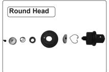
The head can be opened up to access the ratchet mechanism either by releasing the circlip using a pair of internal circlip pliers (fig.1) or removing the securing screws (figs. 2,3 & 4).
