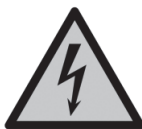
Electrical shock hazard
