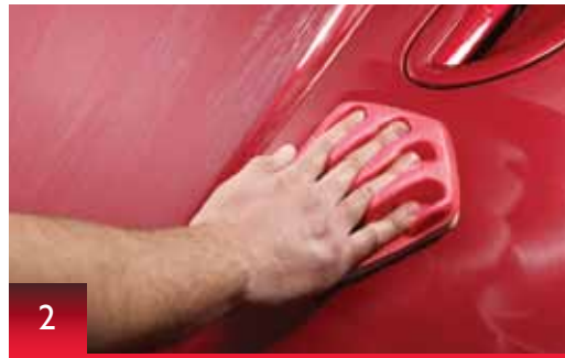
2 Spread the polish on the body with the cloth or applicator and use large circular motions to work the polish in. Treat a small area at a time, then lay this area off in straight lines before treating the next section.
