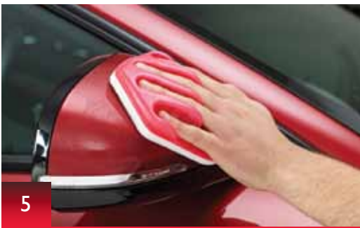
5 Pay special attention to faded paint and plastic areas such as door mirrors and bumpers which are painted with plasticisers in the paint.
