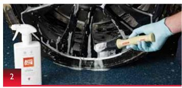
Working on one wheel at a time agitate with the **Hi-Tech Wheel Brush** making sure that you reach all surfaces. Use a thin powerful jet to hose off thoroughly and do not let the cleaner dry before hosing off.
