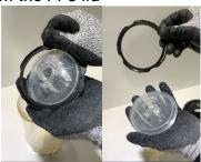
b. (Optional) Remove\* the filter from the inside of the lid
