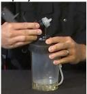
8) Attach the loose end of the air hose to the H/O conversion Pack supply port
