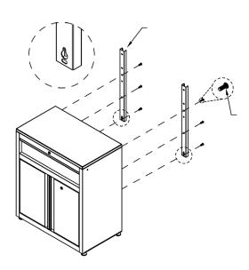
**STEP 3:** Slide 2x peg board rails fully onto the cabinet posts. Place one pegboard on the front, making sure the grommet hole is on the bottom. Attach using 2x M6x16mm screws per rail.
