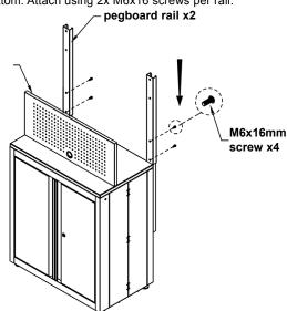
STEP 9: Screw 2x M6 x 16mm into the back of the top cabinet, leaving a 0.8cm. Do not tighten bolts fully. Hang the wall cabinet on the top of the rails, then fully tighten the screws. Attach the bottom of the wall cabinet to the rails using another two M6x 16mm screws.
