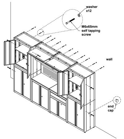
STEP 12: Attach the modular storage kit to the wall using twelve M6x65mm tapping screws and washers insert through wall studs. Insert the 6 end cups on the side panels of the cabinets.
