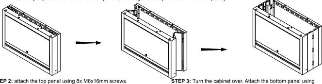
STEP 2: attach the top panel using 8x M6x16mm screws.
