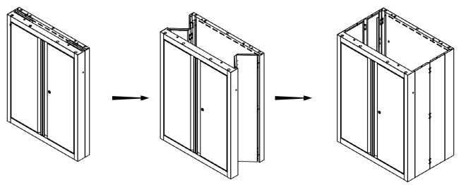
**STEP 2 TOP CABINET:** Attach the top panel using 8x M6x16mm hex socket head screws.
