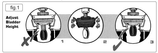
**NOTE:** It may not always be possible to adjust the bladder the desirable position (two thirds of the bladder below lower flange). The flexible nature of the inflatable bladder will create the required seal in these applications.
