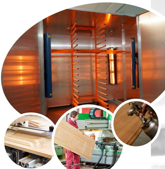
The Heatlight infrared drying system from Victory has been designed to meet the needs of busy manufacturers that need to quickly dry painted or coated wood and metal.
