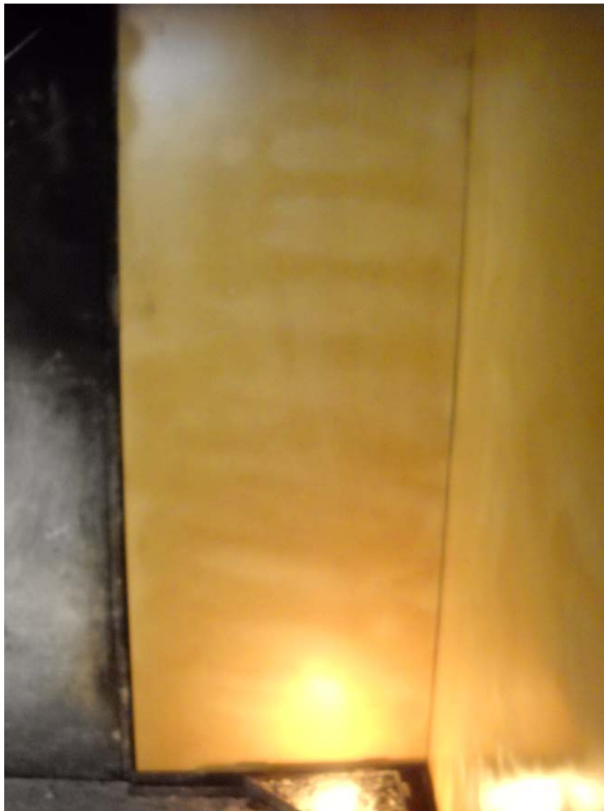
Appearance of the sample before the SBI test (short flap) according to UNE-EN 13823:2012
