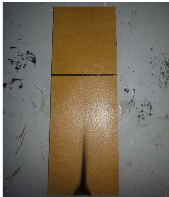
View of the sample after ignitability test according to UNE-EN ISO 11925-2:2011 (applied to edge)
