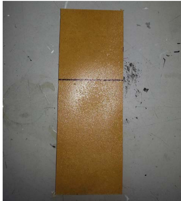
View of the sample before ignitability test according to UNE-EN ISO 11925-2:2011 (applied to edge)
