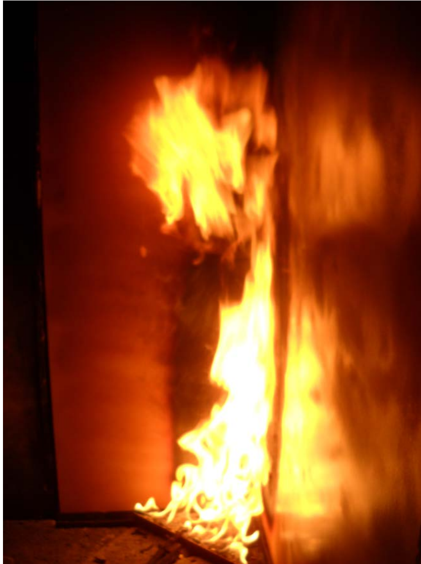
Appearance of the sample during the SBI test according to UNE-EN 13823:2012
