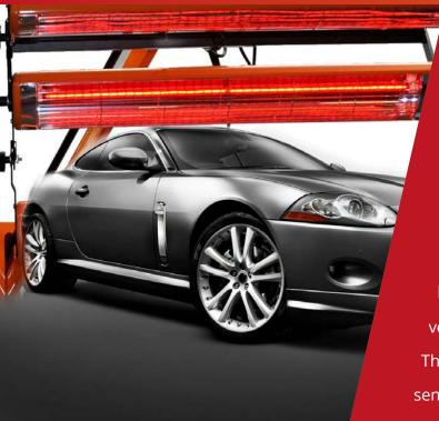
Victory's Heatlight range of large paint dryers utilises 1 & 1.5kW glare control lamps, configured in individual cassettes to yield up to 6kW of drying heat. The lamps emit short wave infrared heat which is ideal for optimising drying of water-based paints. These flexible systems allow each cassette to be adjusted and locked into position around the contours of the vehicle body, ensuring maximum area coverage. There are also options for temperature/distance sensors for ultimate controllability.
