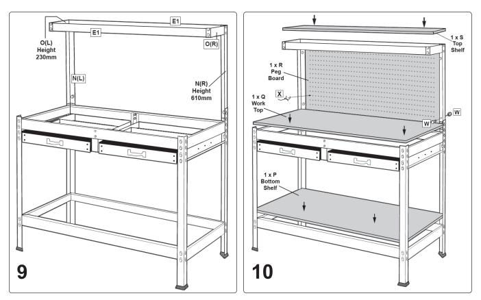
5.5 Attach the extension posts to the back two uprights and assemble and mount the top shelf frame as shown in diagram 9.5.6 Attach the peg board to the back of the uprights and position the top shelf, work top and bottom shelf as indicated in diagram 10.5.7 Attach tool hooks to peg board as required. See diagram 10.
