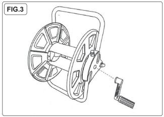
Attach the crank handle through the stand holder (fig.3).
