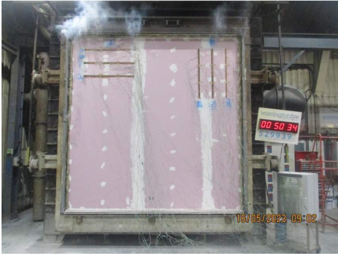
The unexposed face after a test duration of 50 minutes 34 seconds
