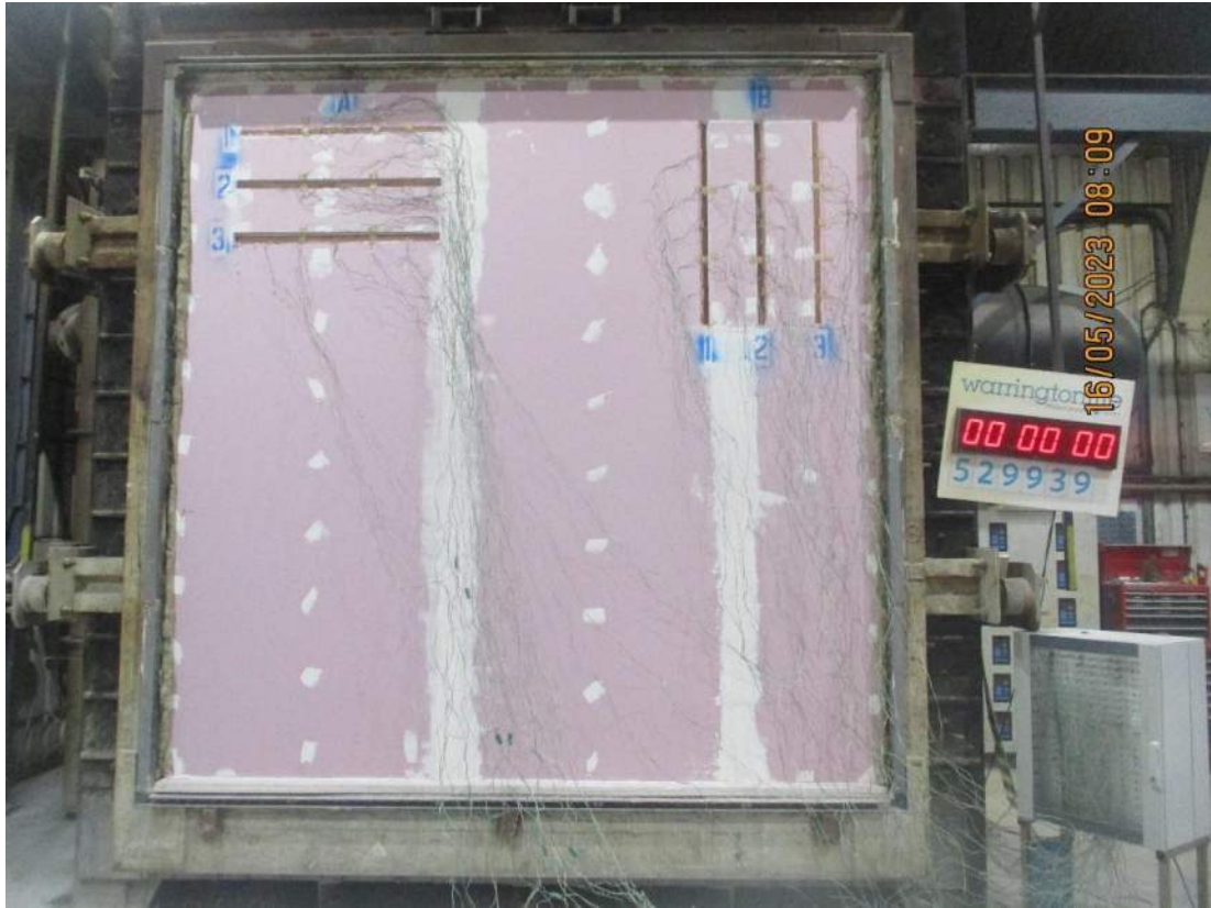
The unexposed face prior to testing
