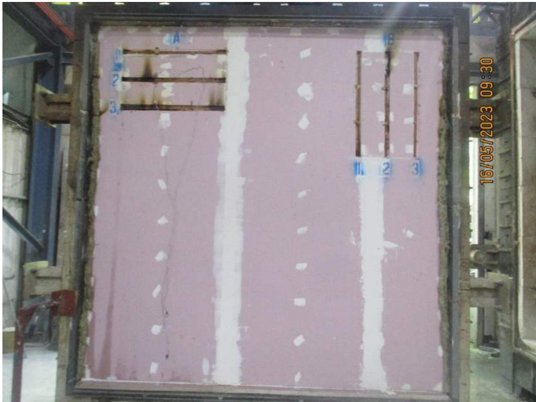
The unexposed face after the completion of the test
